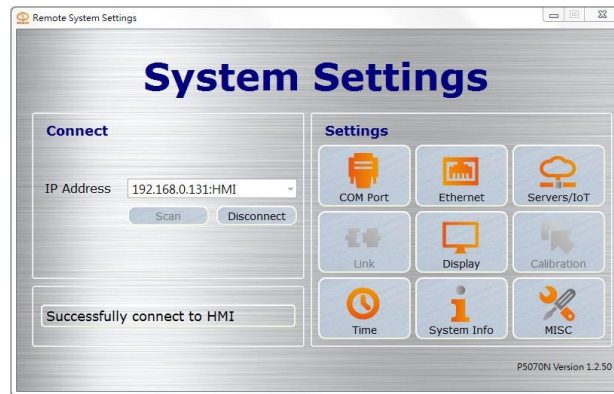
Figure 414 【 Remote System Setting 】 successfully connect to HMI
