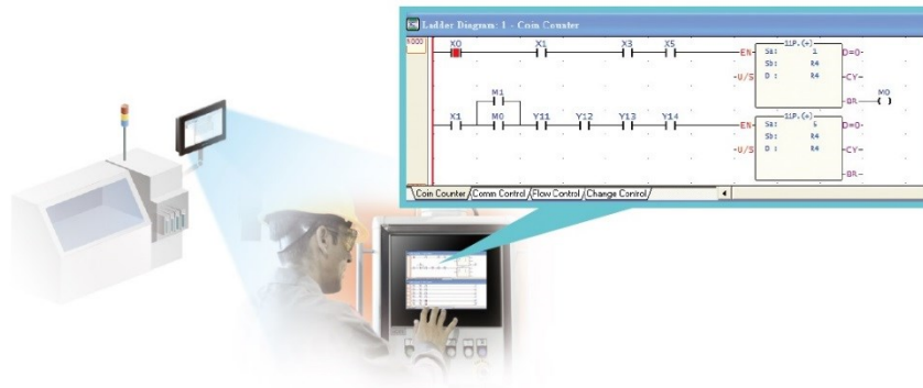
Figure 463 HMI show PLC Ladder Diagram Program illustration
